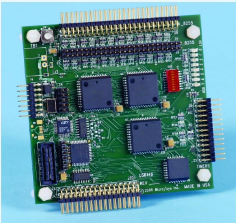
The USB148 is an example of a StackableUSB high-density digital I/O and timer card.
