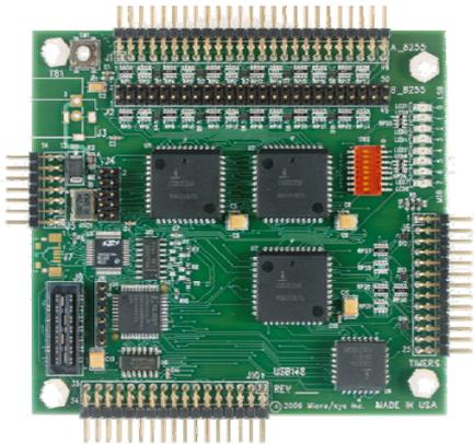
The USB3148 operates as a USB 2.0 Full-speed device in a StackableUSB system or connected to a PC using a standard USB cable. Three (3) 82C55's provide 53 lines of bi-directional general system I/O. An on-board 82C54 provides three (3) counter/timers. There are also two (2) RS232 serial ports, one (1) each I2C and SPI bus interface, a single comparator, and a 10-bit A/D converter. The USB3148 provides this wealth of system I/O on a small 3.55 x 3.755 footprint.
