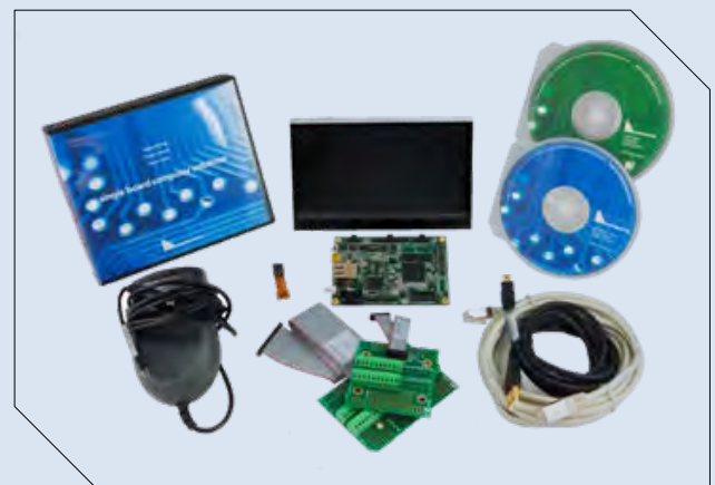
DKV4661 includes SBC4661, cables, sample software
